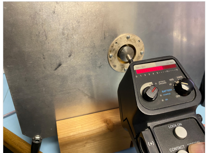
Figure 9. Try to aim for the center of the target as you approach it at 90 degrees during air discharge testing. The newer-style target is much more difficult to hit accurately.
